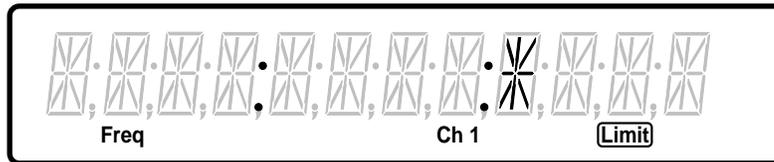
The asterisk is now out of the limits as it has exceeded the entered 10.2 MHz upper limit. (Note the **Limit** annunciator lights since the signal is out of limits.)
