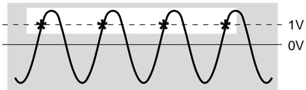
If you want to trigger on the negative (or falling) edge of the input signal, then perform the following step.
