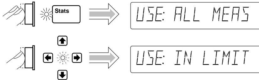
Since the Limits were set to 100 Mega and 102 Mega values that are based on a scale of 10 and offset of 1 Mega, you must re-enable Math now to get the measurements to be within the limits. Perform the following steps.
