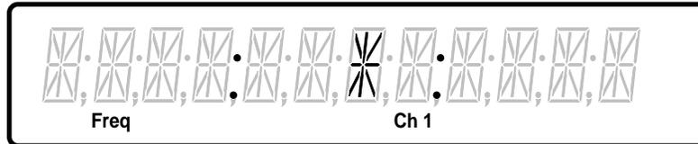
The asterisk represents the measurement and the colons (:) represent the limits you set. This graph indicates that the measurement is within the limits. The colon to the left represents the lower limit, and the colon to the right represents the upper limit.
