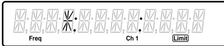
The asterisk is now out of the limits as it is below the entered 9.8 MHz lower limit. (Note the **Limit** annunciator lights since the signal is out of limits.)
